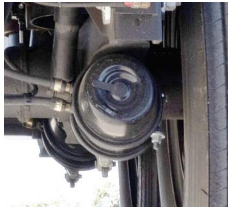
Piston-Type Chambers: High-efficiency piston chambers for reliable and consistent braking performance
