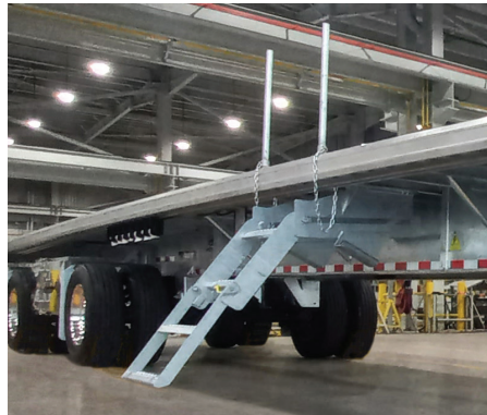
Side Ladder: Easy access to the deck with a built-in ladder for convenience.
